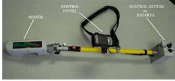
Şekil 3. NTech, GreenSeeker Model 505, spektrometre.
